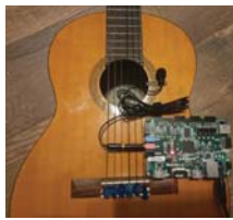
Fig. 4. Testing platform with guitar and FPGA
